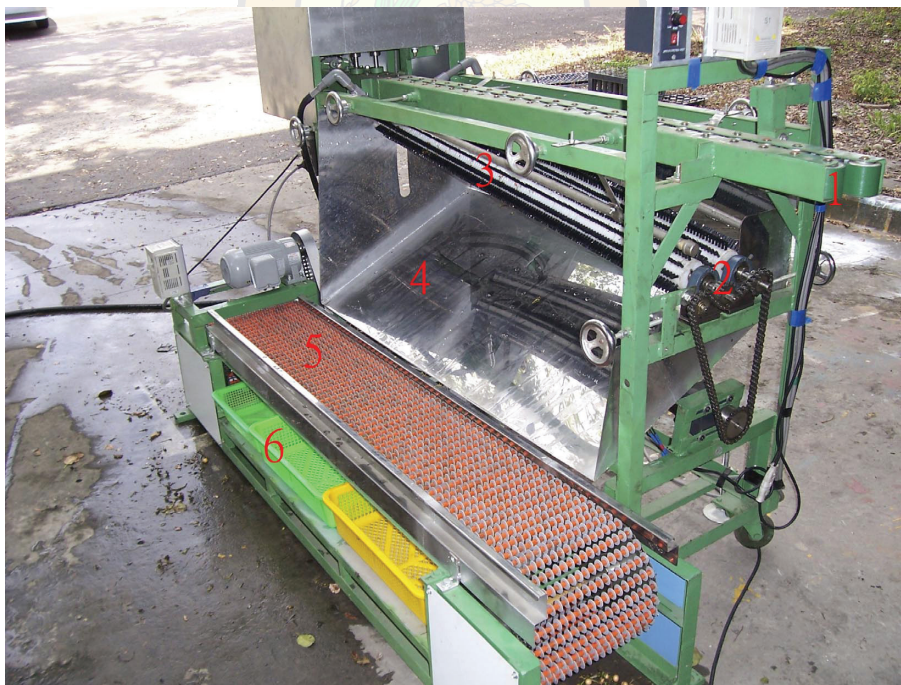
Item annotation : 1. Feeding belts 2. Snapping brush rollers 3. Water pipe system 4. Fruits-collecting chute 5. Screening device 6. Fruits Tray
